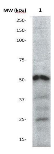
Western Blot: The whole celllysate derived from PDGF stimulated 3T3 was immunoprobed by Rabbit anti-AKT1(pT308) (Cat#600-210) at 1:1000. An immunoreactive band was observed around ~60 kDa.
